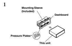
\* If the installed mounting sleeve is loose in the dashboard, the pressure plates may be bent slightly to remedy the problem.
